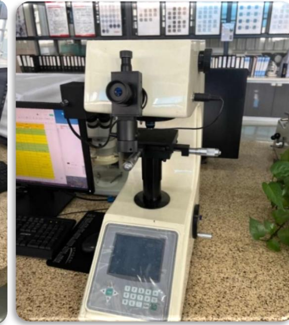
Vickers hardness tester. Testing gradient hardness
