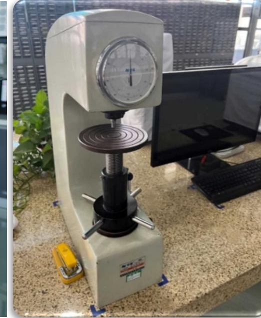
Rockwell hardness tester
